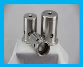
From the <u>Pressure side</u>, when the valve is normally closed and the tank pressure exceeds the rated pressure on the outside of the valve, the valve automatically opens and vents air to atmosphere.
